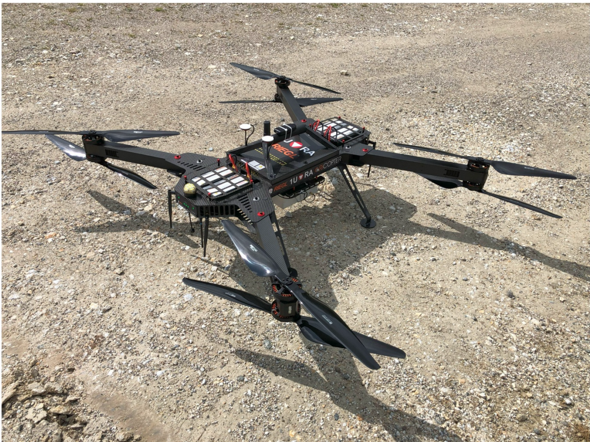
Fig. 8: Drone with payload to monitor strength and direction of multi-wavelength electro-magnet signals. Dimensions of the detector enclosure are 200 by 200 by 100 mm. (Photo by the authors)
