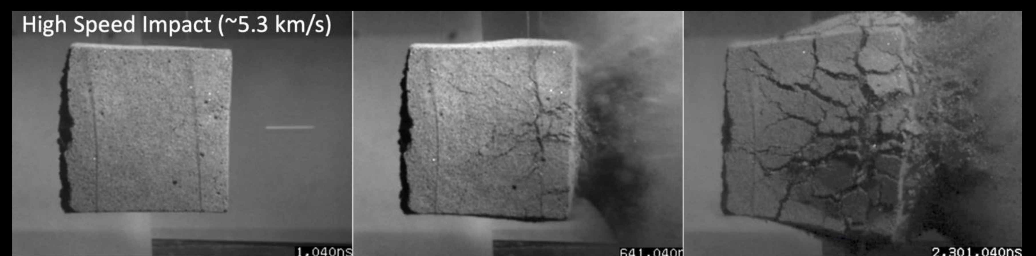
Figure 2. For targets, we use 9 x 9 x 9 cm blocks of CI carbonaceous chondrite simulant prepared by Space Resource Technologies [Metzger+2019] as these are the closest analog to Bennu material [Lauretta+2024]. We conducted 3 head-on impact experiments at 5.3 km/s using aluminum projectiles with diameters, D_p = 3 and 5 mm. These sequence of images over 2.3 ms show the case of a 5-mm diameter projectile.
