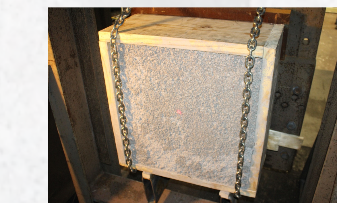
Targets included large hematite rocks in concrete. This hematite rock impacted at 5.33 km/s (LGG-252).
