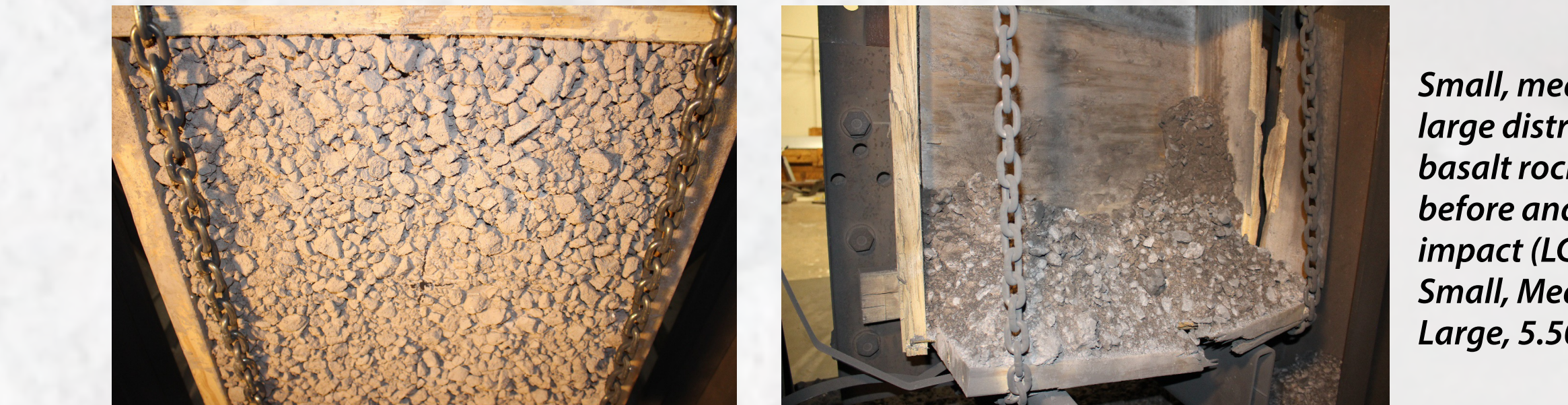
Result of 3-cm-aluminum sphere impact into small basalt target (LGG-403, Small, 5.25 km/s)
