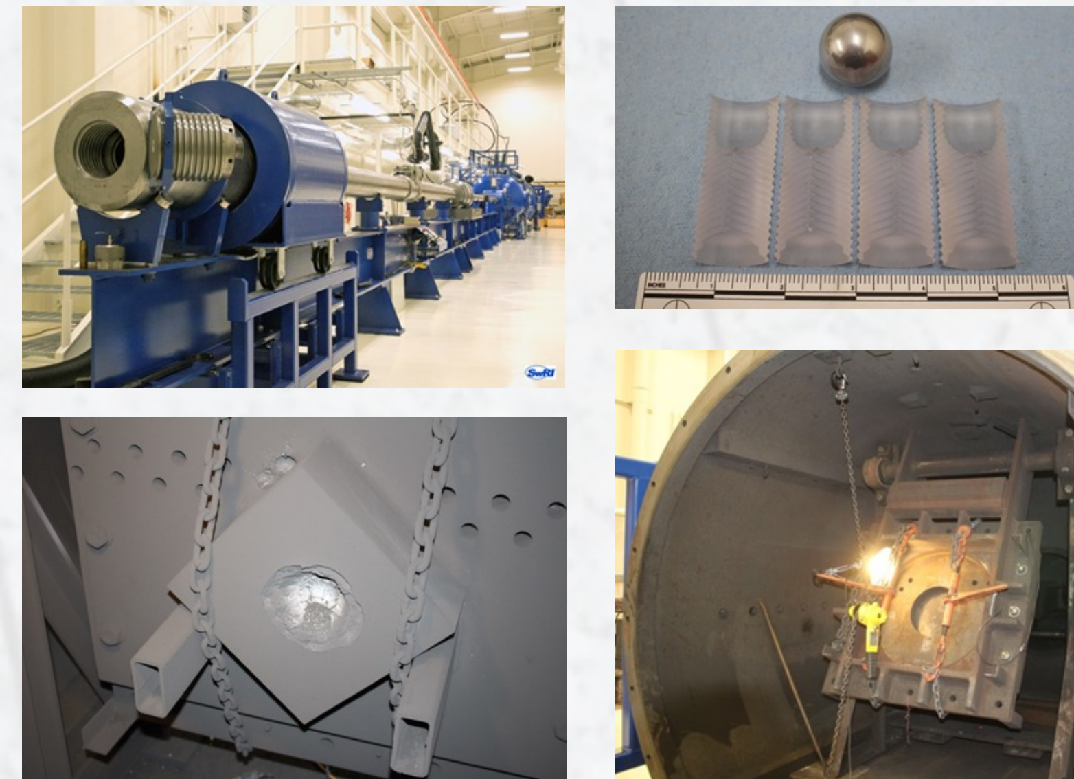
Impact tests at SwRI: SwRI's large two-stage light gas gun, 3 cm Al Projectile and sabot, Al 2024-T351 target attached to ballistic pendulum in evacuated target tank
