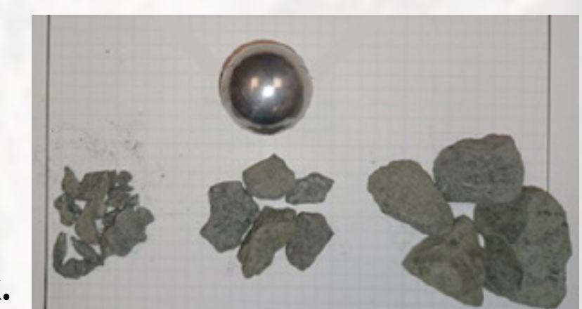
Figure shows 3-cm-diameter aluminum impactor and the three sizes of crushed basalt used in the study.
