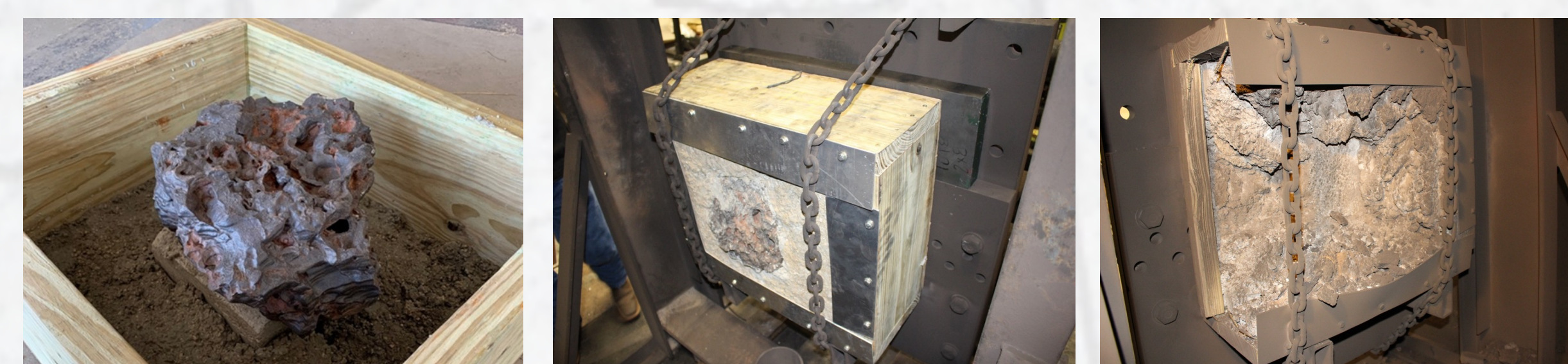
Targets included large hematite rocks in concrete. This hematite rock impacted at 5.33 km/s (LGG-252).
