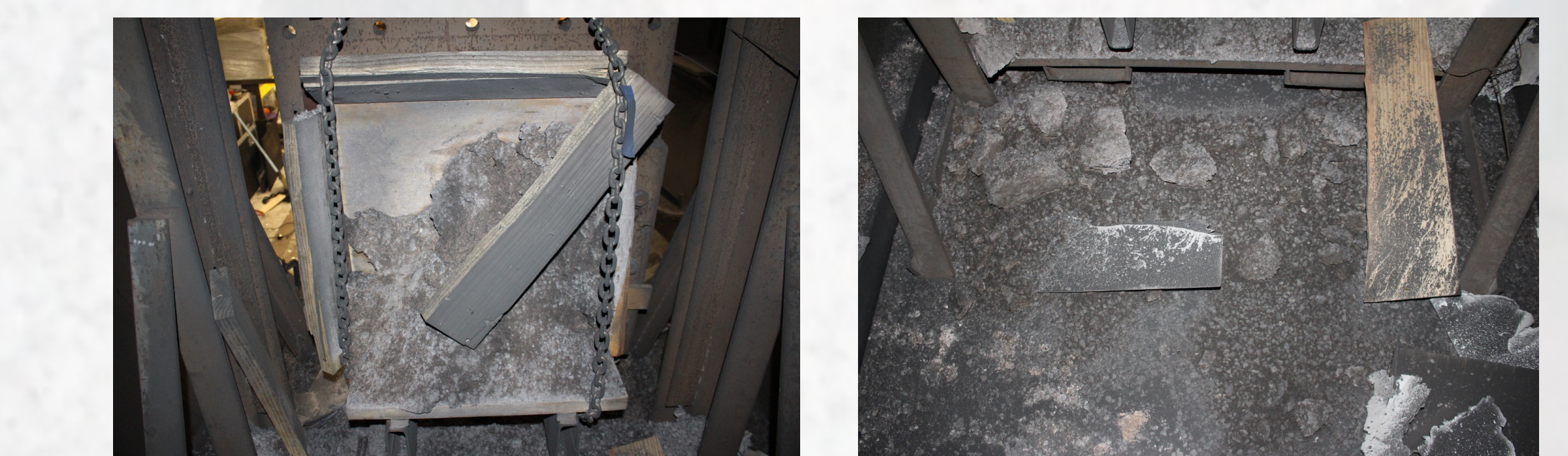
Result of 3-cm-aluminum sphere impact into small basalt target (LGG-403, Small, 5.25 km/s)
