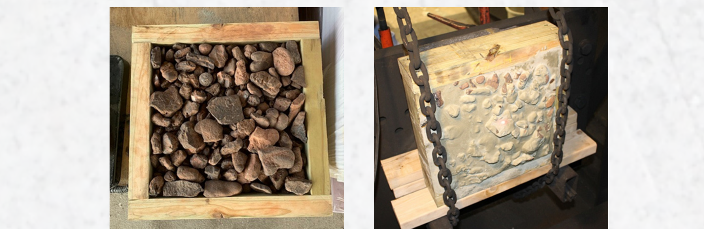
Targets included large hematite rocks in concrete. This hematite rock impacted at 5.33 km/s (LGG-252).
