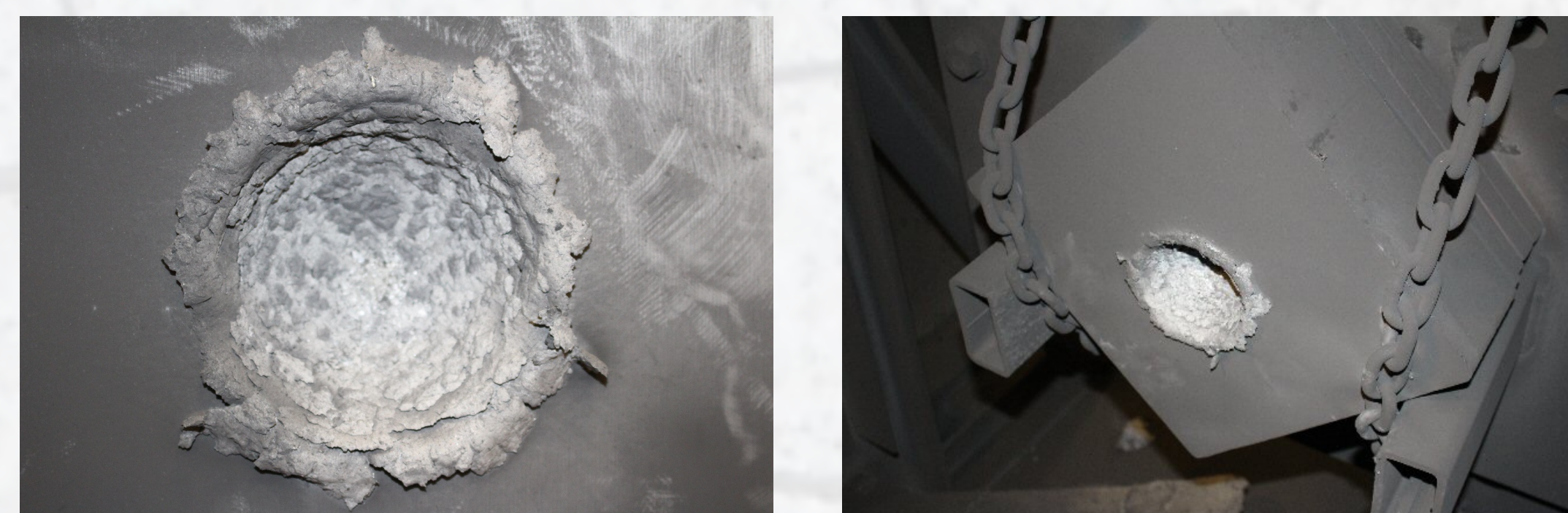
ARMCO iron (pure iron) target struck at 4.81 km/s (LGG-248)
