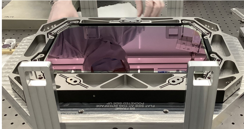
Figure 6. Flight spare beamsplitter frame assembly, prior to removal from bonding fixture
