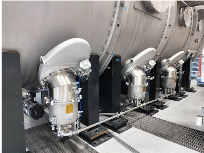
Figure 15. New TVAC chamber in commissioning process at SDL to support NEO Surveyor
