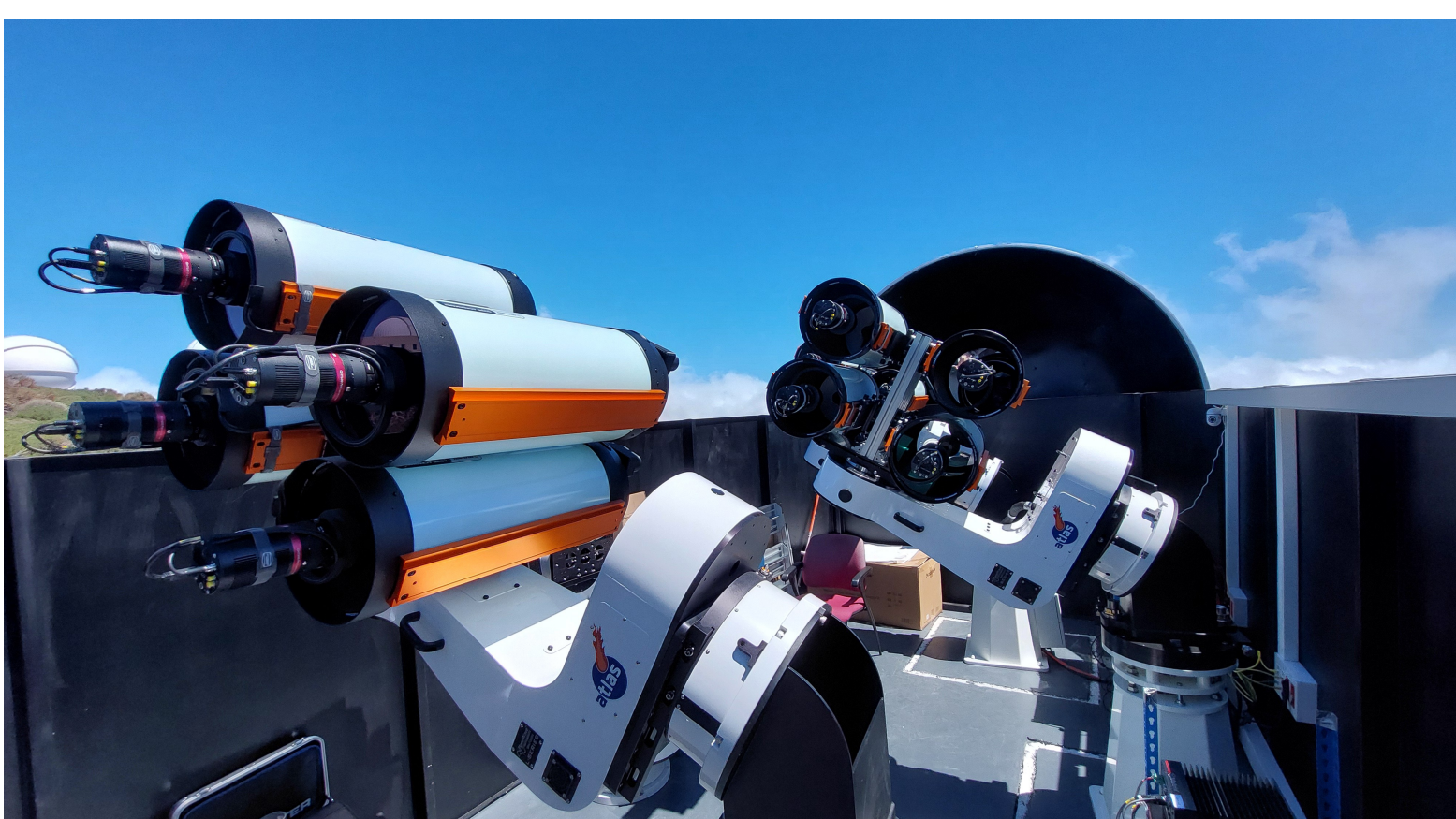
Two of the 4 ATLAS modules installed at Teide Observatory.
