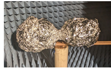
Figure 4: Image of an anechoic chamber model of a fused binary shaped asteroid
