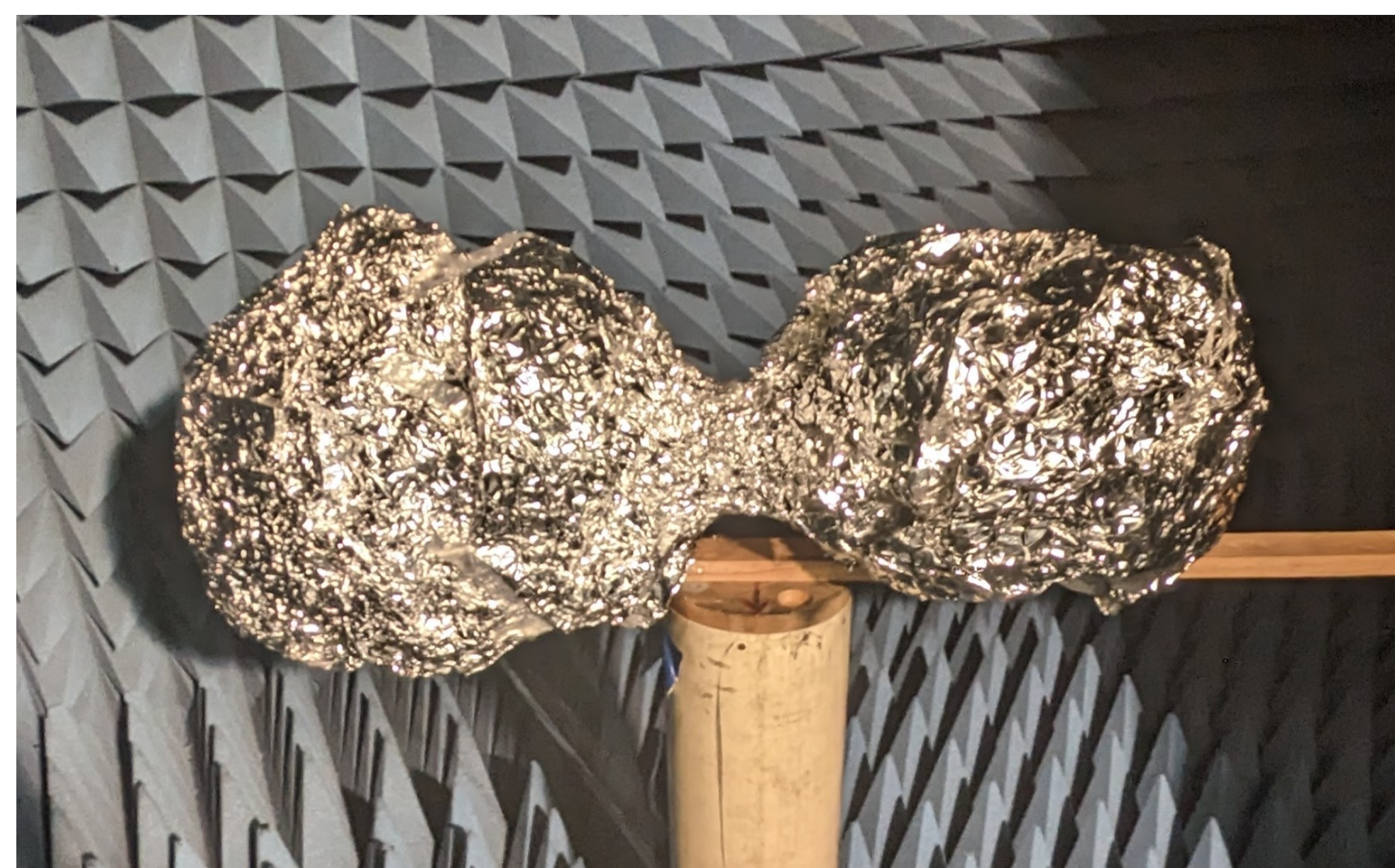
Figure 4: Image of an anechoic chamber model of a fused binary shaped asteroid
