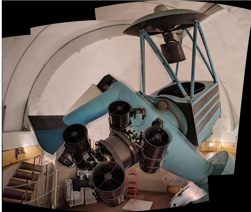
Figure 1: A panoramic view of the “Cassini” telescope and the TANDEM array. “Cassini” is on the right, while TANDEM is the array of 4 telescopes on the left.
